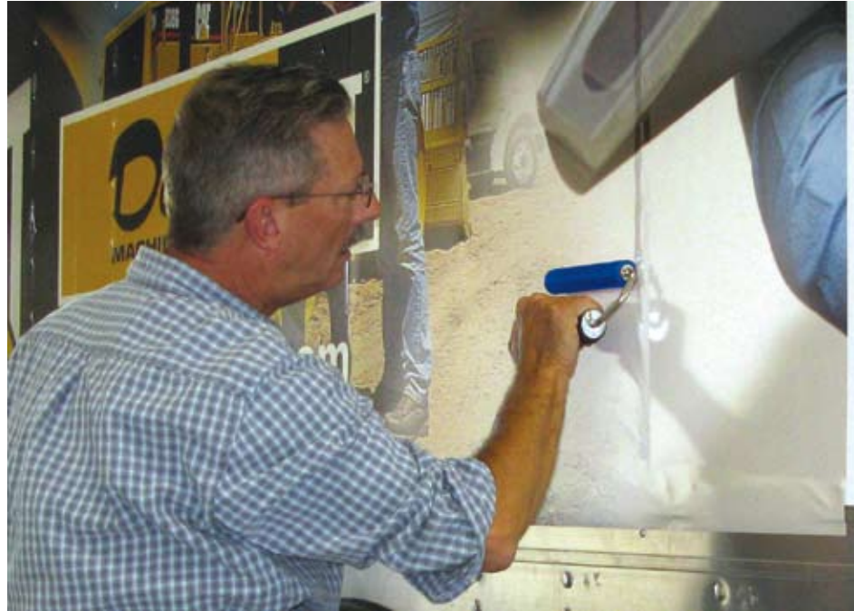
Rob demonstrates a rolling technique with 3M's Power Grip Rapid Roller CPA-2, a rolling tool that facilitates applying vinyl over riveted surfaces. He emphasizes the importance of mastering new tools and techniques to make your shop more efficient.
