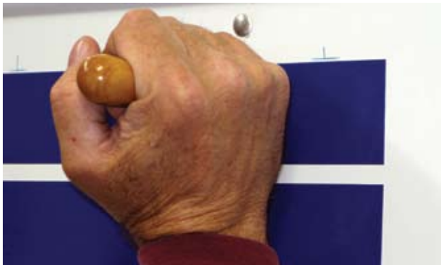
After letting the vinyl cool, use a rivet brush until air has been released. According to Rob, three or four passes are usually required for each rivet. Once most of the air has been released, center the brush atop the rivets, and brush firmly in small, tight circles.
