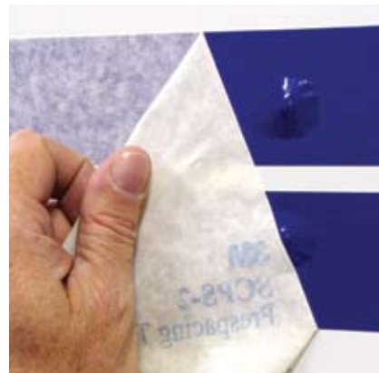
The result of a successful squeegee process – a small air pocket encircles the rivet.
