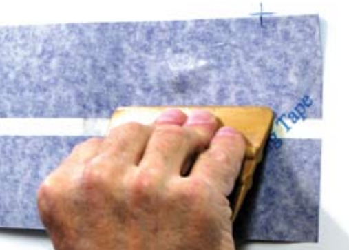
To properly use a squeegee over rivets, make sure the graphic is taut, and roll the squeegee from the middle out in all directions. Also, keep it low and flat.
