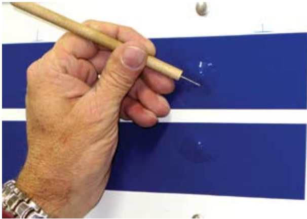
To expel air, use an air-release tool to poke a single, small hole underneath where the rivet meets the surface.
