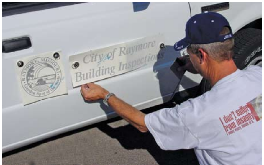
Applying magnets to the graphic while using the hinge method lets the installer use both hands to squeegee and peel.
