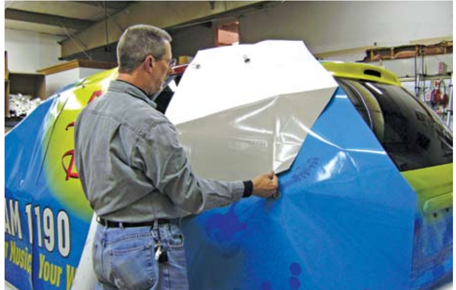
This month, I'll illustrate the various hinge techniques that can be used for vinyl application. Here, I use magnets to hold the release liner as I pull away a large vinyl panel.
