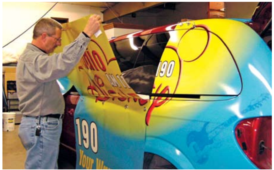
I used a center hinge to install this vinyl section.
