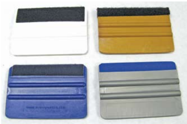
Examples of different edge coverings that help ensure smooth squeegee edges (clockwise from top left): a Lidco plastic squeegee with a felt edge; a 3M Gold nylon squeegee with a Velcro® tip; a Lidco nylon squeegee with an edge covered with Bondex pressure-sensitive nylon; and an Avery nylon squeegee with a blue-felt edge.
