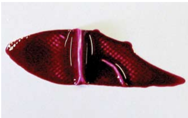
3M printed this small vinyl sample on Controltac® film using a Roland DGA Corporation printer and Eco-Sol Max ink. The printer applied only two ink drops, and the sample cured for only five minutes before lamination.
