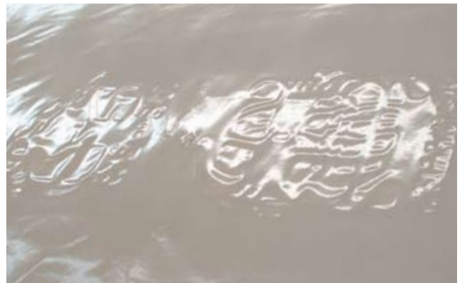
This sample, which also contains Controltac film and Eco-Sol Max inks, cured for 72 hours and laid flat on a table. The liner was removed to show the vinyl's adhesive side. The solvents have swollen from the printed area.
