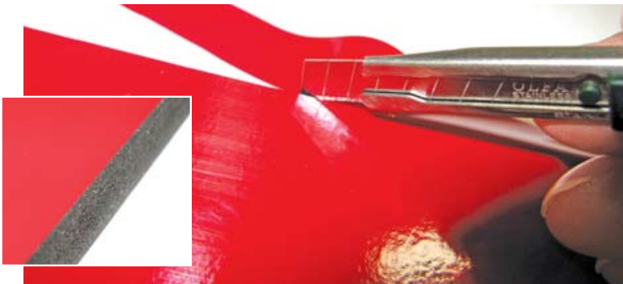
Note the small black color on the blade's tip – it's a reflection of the black substrate. This indicates the flat edge isn't touching, and the beveled cutting edge is flush. The close-up shows the perfect, flush-edge trim.
