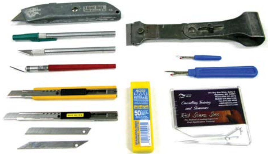
My collection of cutting tools. In the lower left, I've displayed two types of Olfa knives and two Olfa blades with different angles. Also shown in the photo are a Zippy letter opener, a seam ripper and a razor scraper.
