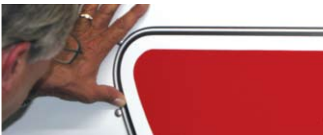
For very narrow stripes, tack the film in place with your thumb. And, of course, remove the clear premask first. Otherwise, it will cause the film to crack.
