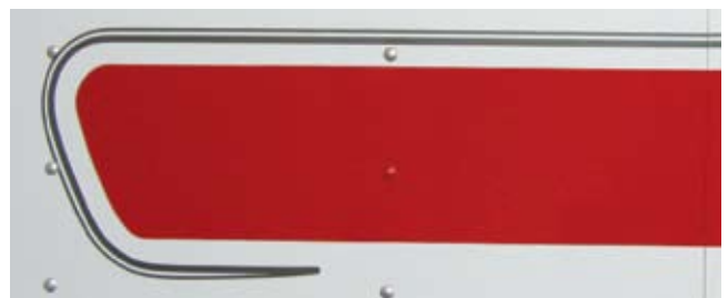
The finished application. For customers who can't afford a vehicle wrap, or who need a cost-effective solution, roll striping provides an effective alternative.
