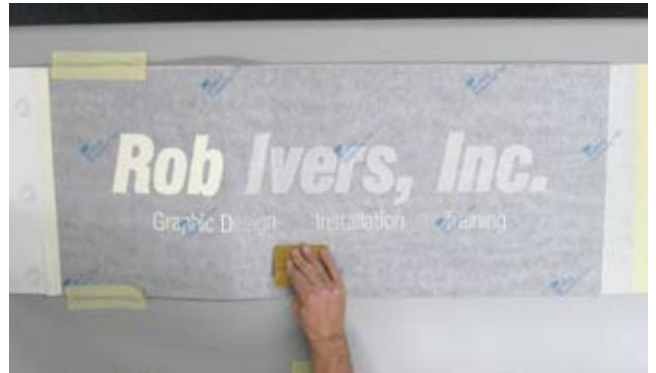
Using the outside edges for placement, I align the black vinyl. Using the side-hinge method, I remove the liner and squeegee right to left, and up and down from the middle.
