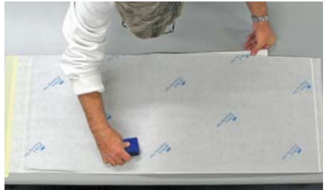
The liner prevents contact with the vinyl as I squeegee up and down from the middle, which expels the air.
