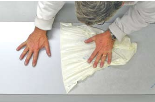
Removing the premask at a 180° angle prevents vinyl lifting.
