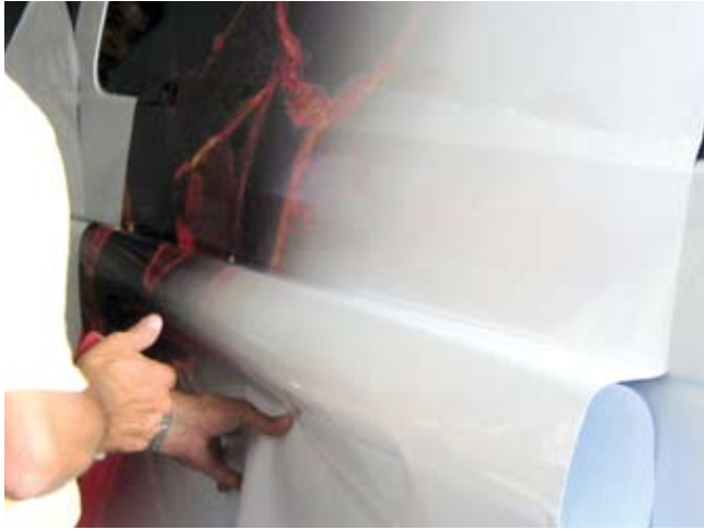
When using a squeegee, work right up to the indentation. Lift the vinyl so it doesn't touch, and give it some slack to avoid stretching.
