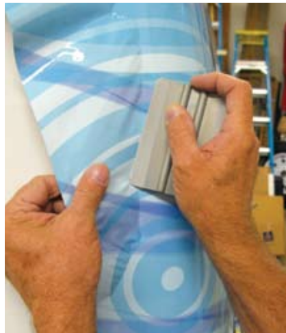
The same piece moments later; note how the heat relaxed the puckers. After it cooled, I began spreading the excess evenly – in this case, up and then down. This technique reduces stretching to a bare minimum.
