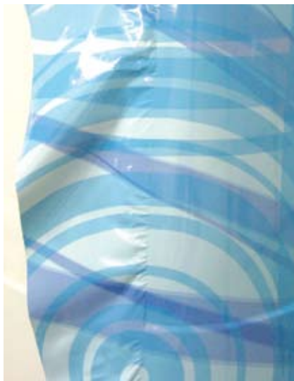
A close-up look of a Ford van's complex curves. To this point, no heating or stretching has occurred. I'll add some heat while the vinyl is loose to relax the film.
